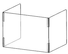
**STEP 3:** Use the adhesive-backed T Shaped Gripper Connectors (included) to attach barrier securely to desktop. Install one in the middle of the bottom edge of each panel.
